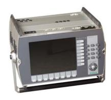
Using current booster module can expand current generation range up to 120A.
